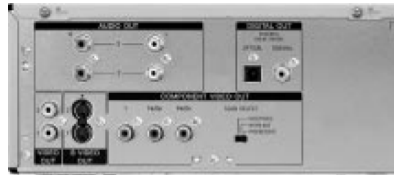
Photo 2: Widely spaced Y/C B /C R output jacks accommodate even extra-fat videophile connectors.
